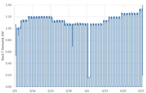
The evaluator used the power factor of the entire lighting panel to approximate power factor at Rack 7. The peak demand at Rack 7 was 1.38 kW for two fixtures. This peak period occurred at the end of the meter period while the site contact set the Rack 7 fixture lighting output to peak. This comes to a peak output wattage of 690.8W/fixture which is within 1% of the rated (peak) input wattage of 685W.
