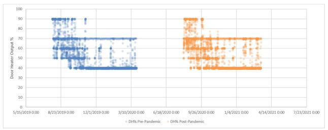
Figure 5-3. Cooler C Hourly Door Heater Percentage Output
